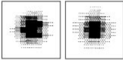
Fig. 1. Restoration of an image distorted by the transposition of rows. The left panel shows one scanned stellar image - the rows’ displacement is probably due to the inertness of the scanning machine. The right panel demonstrates the same image but treated with the first smoothing level of the wavelet transformation
